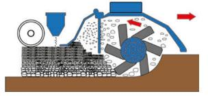
the rear field roller. With the optional seeding unit you are able to make a ready lawn surface on one pass. Stone burier is most commonly used when the topsoil needs to be milled thoroughly.
