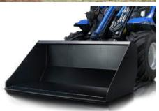
The MultiOne bucket design enables good visibility to the cutting edge, making loading, grading, and dumping more efficient. Length of the bucket has been optimized in order to give best possible breakout force. Heavy duty steel construction includes reinforcement plates inside, slide wear bars on the bottom of the bucket, and the cutting edge is designed for bolt-on teeth.
